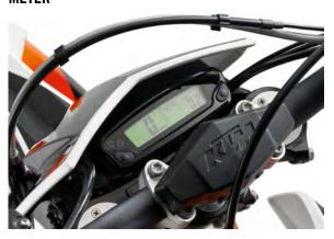
Speedometer from Trail Tech with standard enduro functions + integrated indicator lamp
