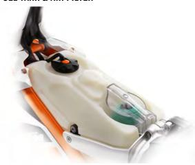
Light weight polyethylene design allows the rider to see the fuel level
